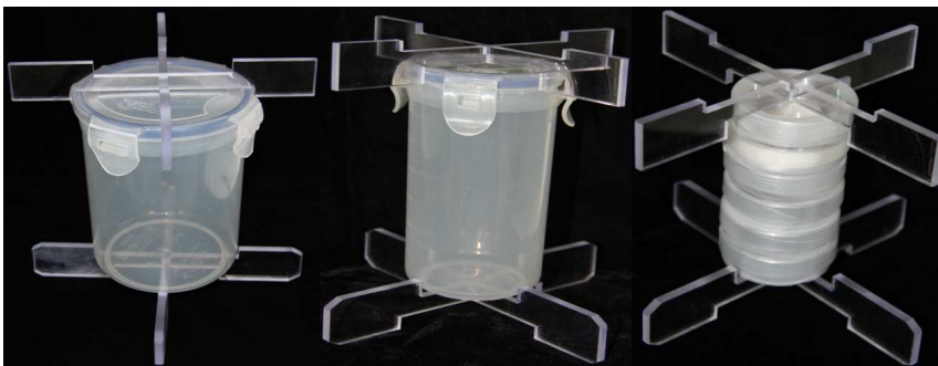
Figure 4: Brackets of varying sizes to fit different sample containers (0.7 litres, 0.4 litres and Petri dishes), brackets are cut from 5 mm PMMA
