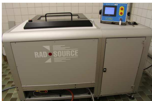
Figure 1: X-ray irradiator RS-2400, sample canisters are loaded and unloaded from the top,
