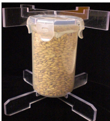
Figure 5: Seed sample packed inside a contained and fixed in place using tissue. The container is fitted with brackets.
