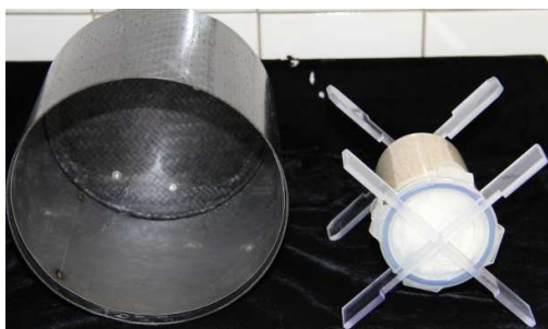
Figure 6a RS 2400 standard sample canister (left, 3.5 litre volume) and a sample container with adaptors (right, 0.4litre volume).
